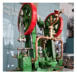
The Swing Bridge is powered by hydraulics to make it spin. You can see one of the original steam pumps from this mechanism at the Discovery Museum.
